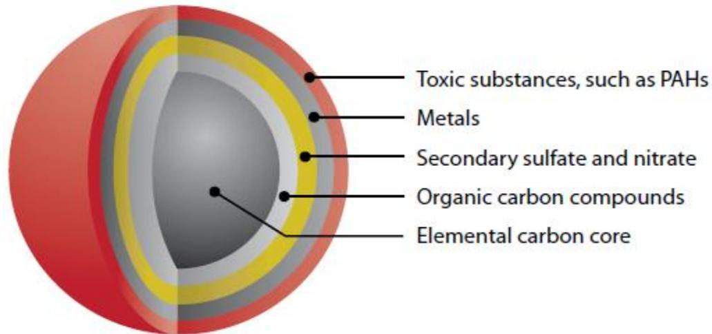
*Elementary composition of diesel particle. Source: NWS DECC, 2008*
